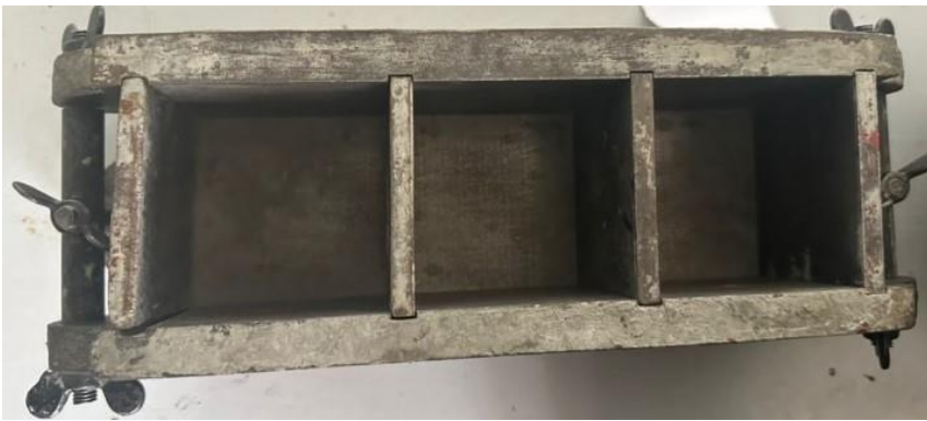
Figure 3: Gang Mould for the Composite Production
